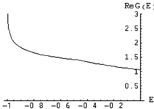
Fig. 1. Real part of Green’s function for the perfect FCC lattice.
